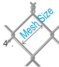
**"Knuckle" design to avoid sharp ends; "Twisted" method for more security.**
